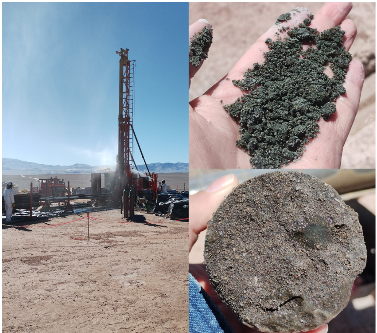
Figure 3. Top – Drilling rig set up at K25D44; Upper right – fine grained sand sample typical of the drillhole bgs; Lower right – fine grained sand from 606 m bgs
