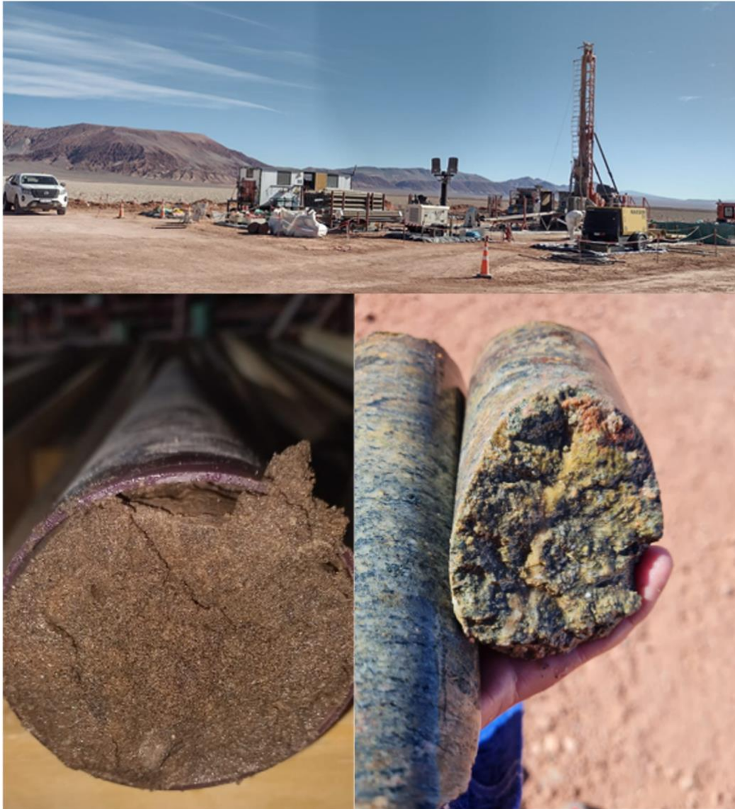
Figure 2. Top – Drilling rig set up at K24D41; Lower left – fine grained sand sample from 455 m bgs; Lower right – metamorphic basement rock encountered at 595 m bgs
