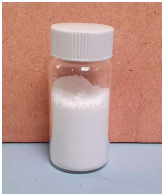
Figure 19: Lithium carbonate (battery grade) produced by Lilac IX process
