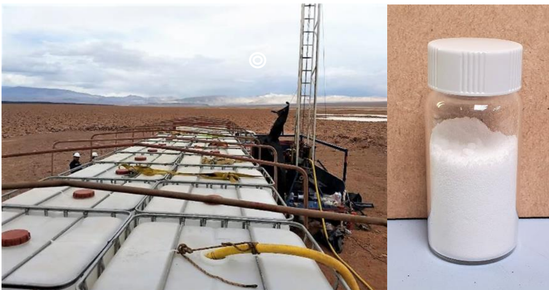
Figure 2: a) Lithium bearing brines pumped into containers at the Kachi Lithium Brine Project for trucking to port for dispatch to California; b) Lithium carbonate product with 99.9% purity and low impurities from the Kachi Lithium Brine Project using Lilac's direct extraction ion exchange process.
