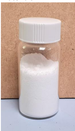
Figure 1: Lithium carbonate product with 99.9% purity and low impurities from the Kachi Lithium Brine Project using Lilac’s direct extraction ion exchange process.
