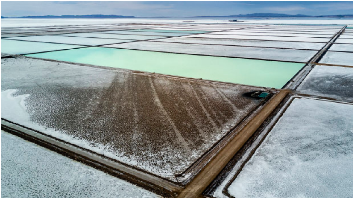
Lithium brine production traditionally employs giant evaporation ponds to extract lithium carbonate.
