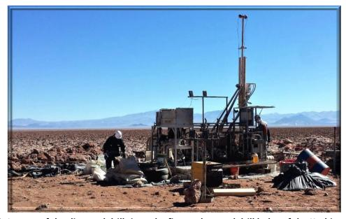
Fig 2: Images of the diamond drill rig at the first and second drill holes of the Kachi project
