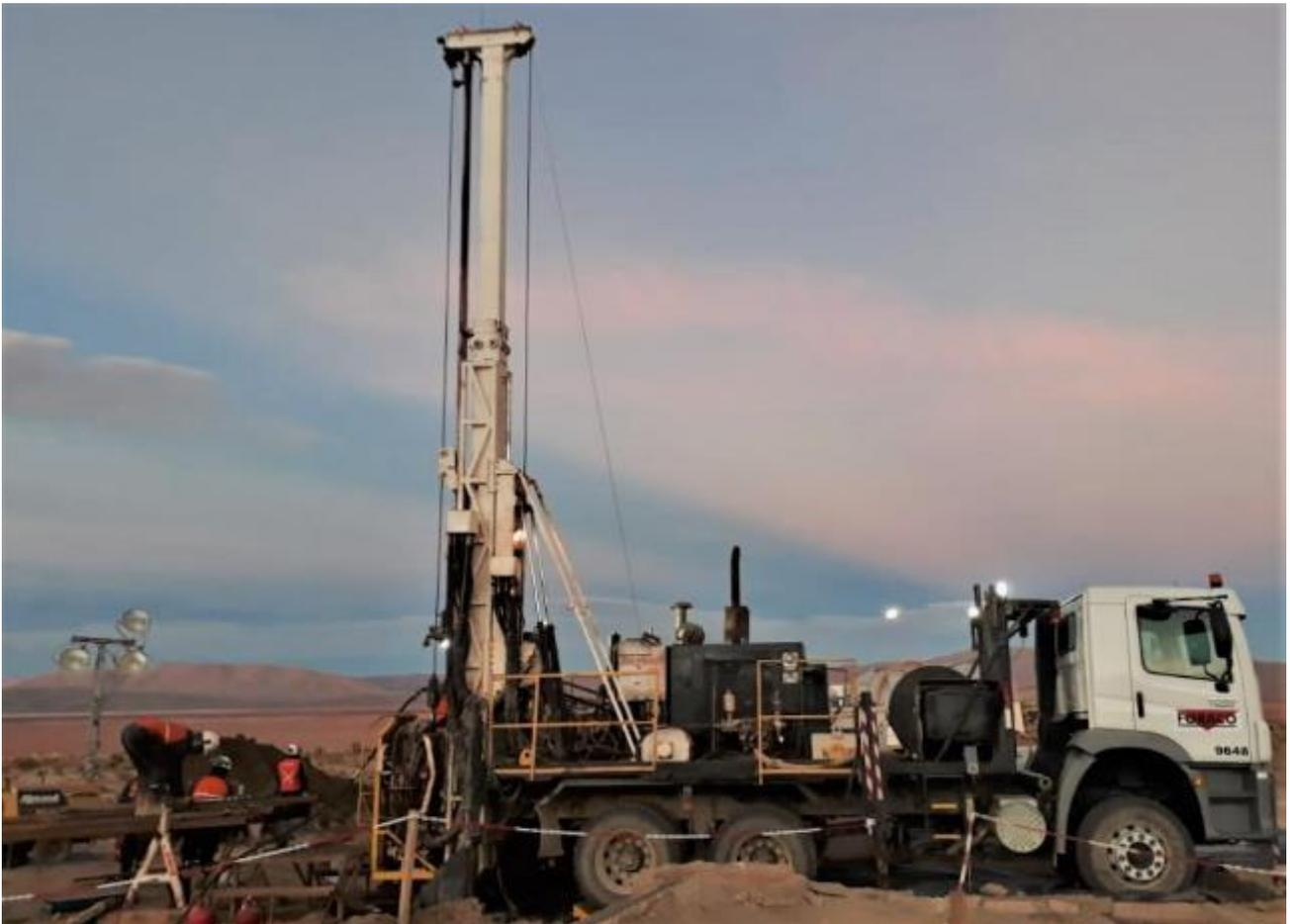
Figure 3: Diamond rig currently operating at site and at 141m deep
