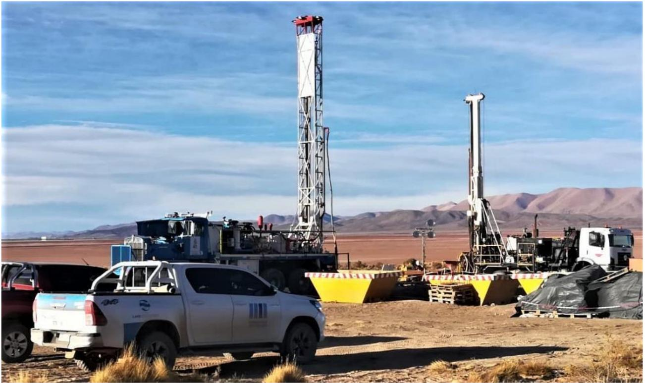
Figures 1: Foraco diamond drill rig (right) next to rotary rig (left) at Cauchari, looking across salt lake to Ganfeng/Lithium Americas project
