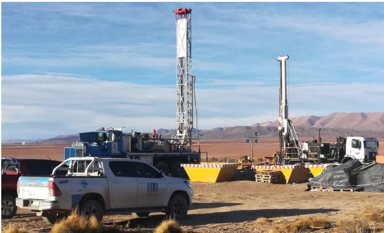
Figure 4: New diamond drill rig alongside the Rotary rig
