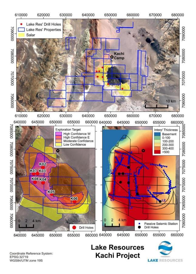
Figure 4. Kachi Lithium Project showing mining lease boundaries and areas defined by levels of confidence to the exploration target and Seismic Survey Results.
