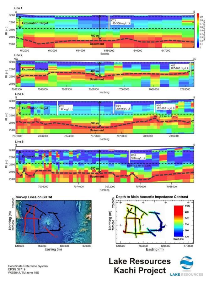
Figure 3. Kachi Lithium Project Seismic Profiles showing location and depth to basement together with the depths used in the exploration target calculation (Red line is the basement reflector)
