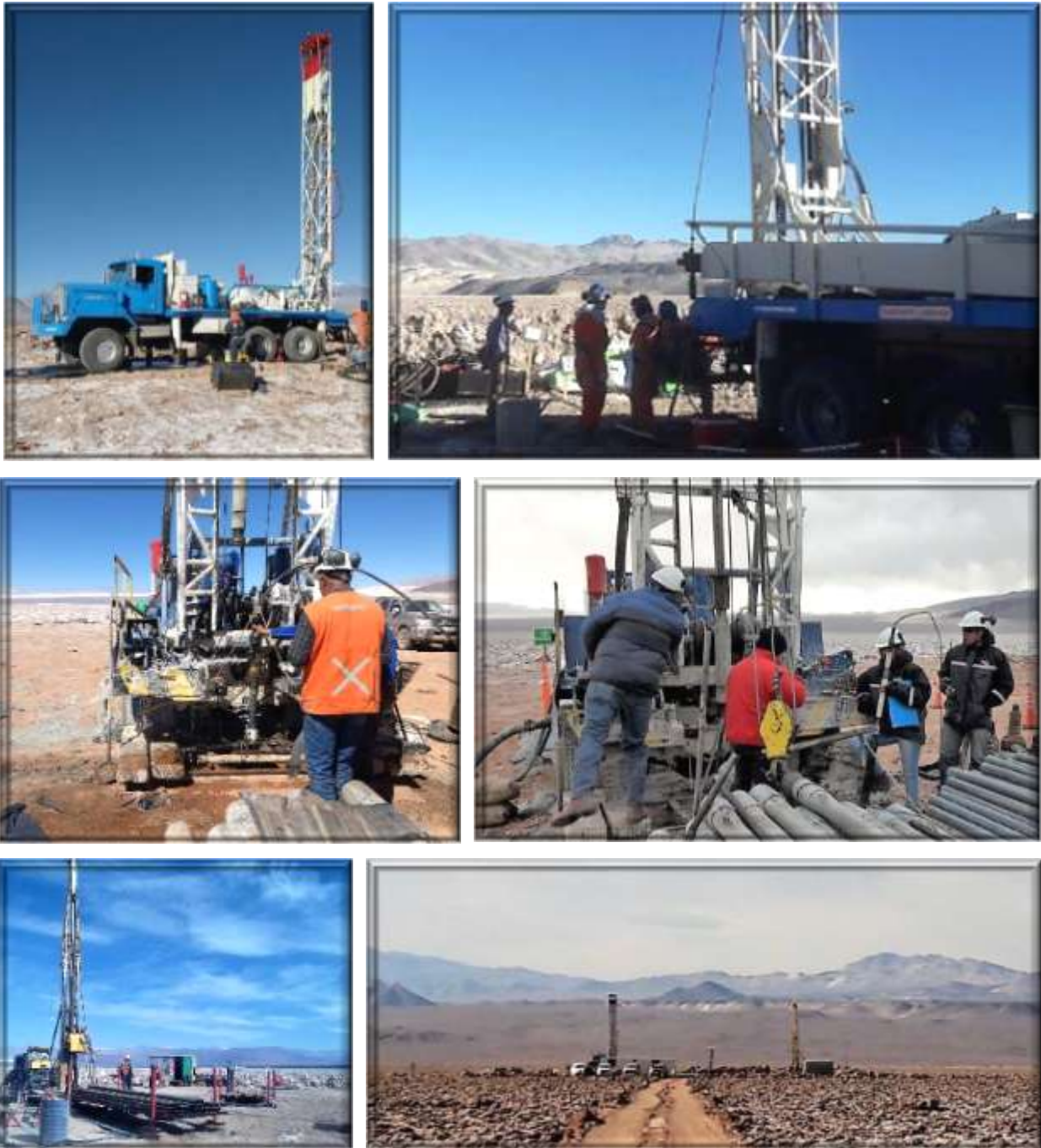
Figure 3: Images of the larger rotary drill rig in the south east of Kachi; the recent rotary drillhole undergoing testing and geophysics in the west of Kachi; the diamond rig in the south east and side-by-side of the rotary and diamond rigs and an indicative map/image of the Kachi project
