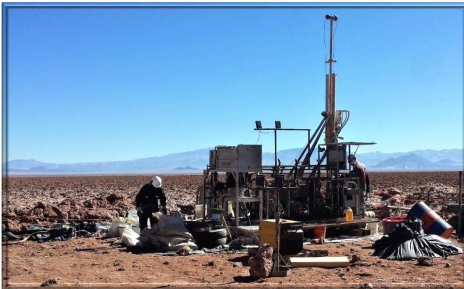
**Fig 2: Images of the diamond drill rig at the first and second drill holes of the Kachi project**
